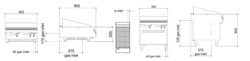
The unit can be connected at the rear or from below
